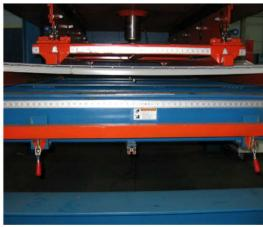
Apply an increasing load up to the point at which deflection of D/165 is achieved. Record the capacity exerted as W1.
