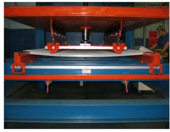
Continue to increase the load until structural collapse occurs. Record the capacity exerted at failure and divide it in half and record that number as W2.
