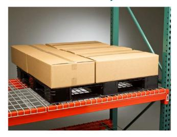
Definition 3.1.15 – Any static load which is evenly distributed over the entire surface on the rack deck independent of the support system
