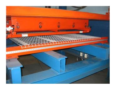
Nashville Wire has an onsite test stand in TN to check the capacity ratings on decks.
